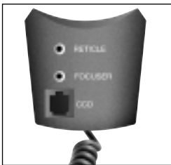
Fig. 19: #909 Accessory Port Module (APM).
