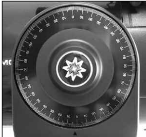
Fig. 31: Section of Declination Setting Circle.
