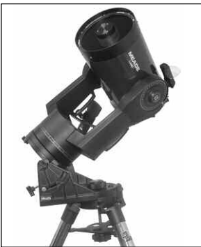
Fig. 32b: LX90 mounted on an equatorial wedge.
